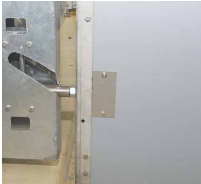
Quick.gate - the built-in mechanism lifts the gate out of the straw.
