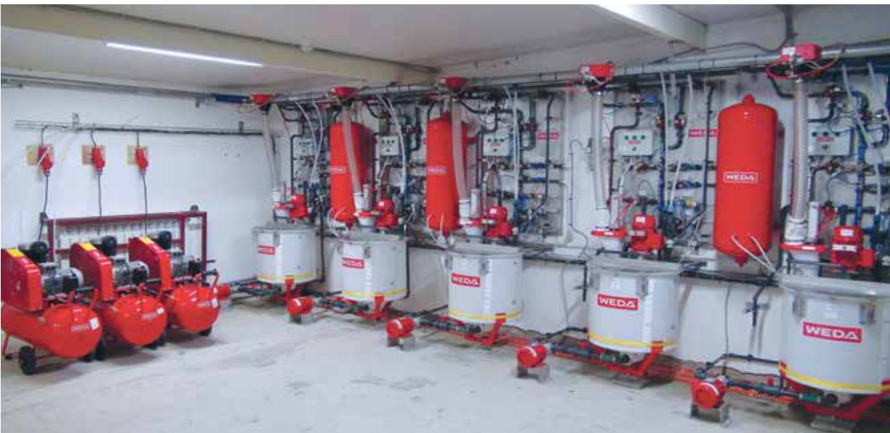
Parallel running system for 2,500 sow places (system can be extended to up to 4,000 sow places).
