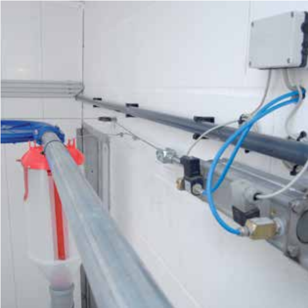
Automatic release mechanism (pneumatic) for volumetric dispensers
