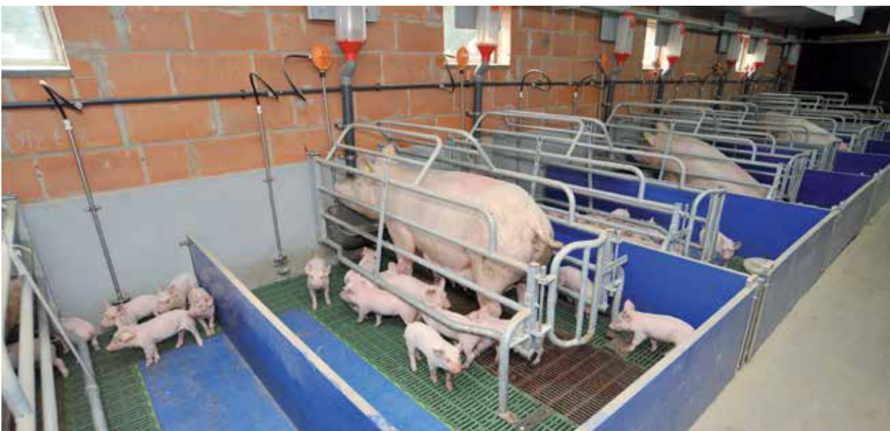
Piglet protection cage AKH: Mounting is possible free-standing, on the wall or on single or double frames.
