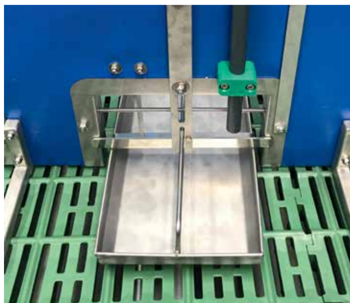
Changeable Nutrix troughs in the sizes small (left) and big (right) allow a smooth transition for the piglets.
