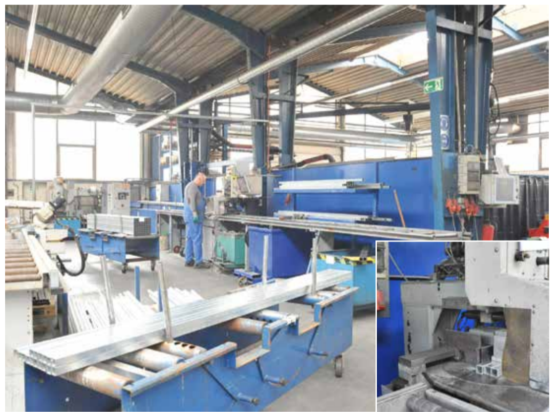
Each square pipe is custom-cut.
