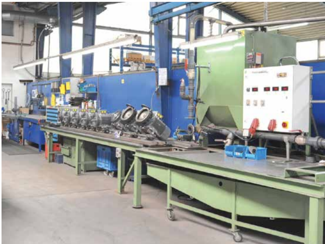
Here, all pumps are tested comprehensively before being sent out to the customers.
