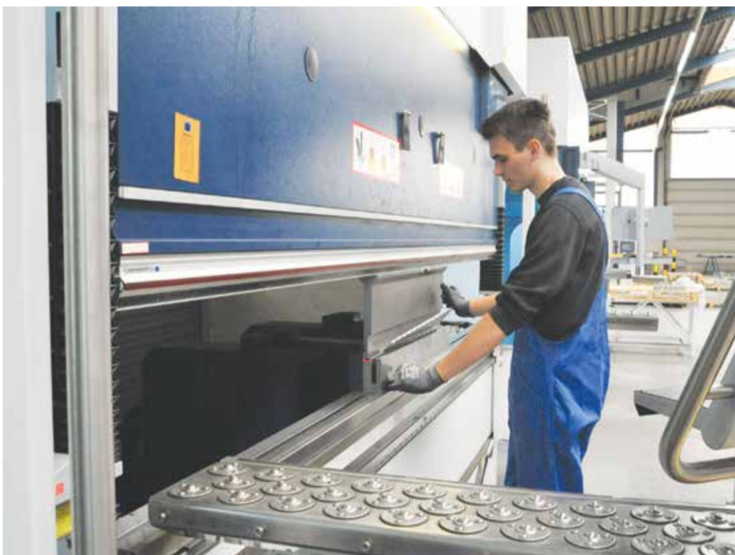
The laser-cut parts for the troughs are shaped at the bender.
