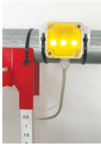
Smart.Light: indicates the current feed intake status of the sow and is controlled via the 4PX.
