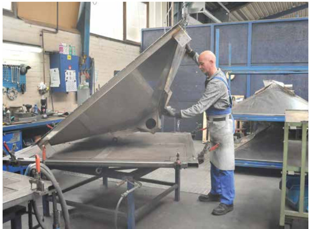
Welding of tanks for WEDA liquid feeding systems
