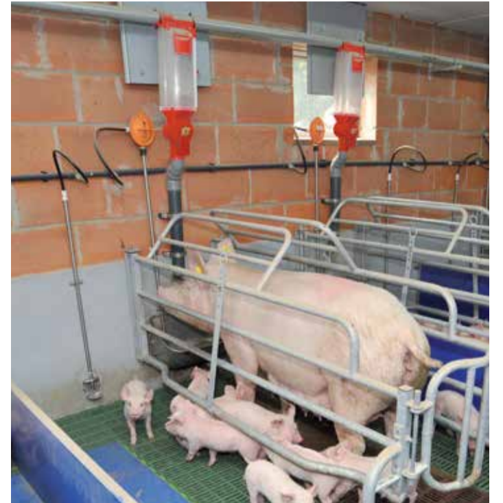
Any existing dry feeding system can easily be equipped and retrofitted with the OptiMum system: it is simply installed below the volume doser and regulates feed dosing according to the sow's individual requirements from there.
