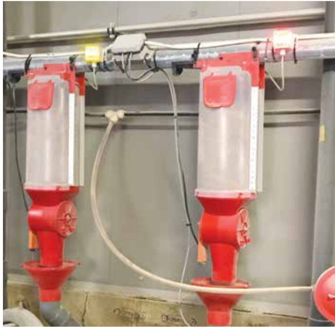
Smart.Light shows the stable staff directly whether the animal has consumed sufficient feed.
