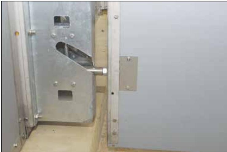
WEDA Quick.Gate: the hinge lifts the gate out of the straw by itself.
