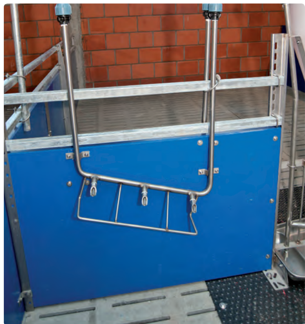
Circuit pipe for three drinkers
