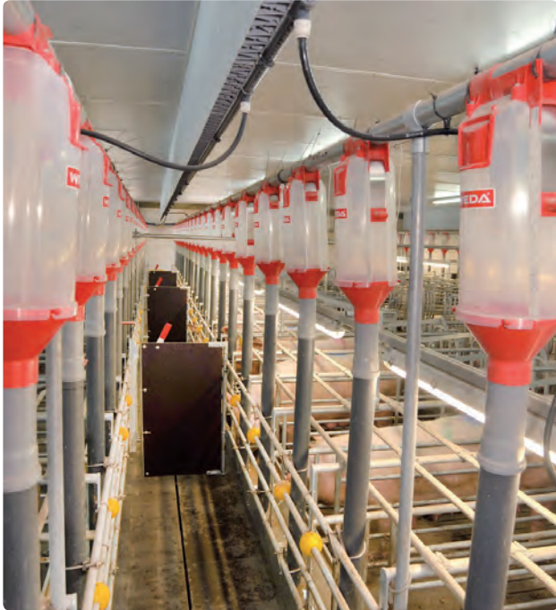
Volume dosificator for one feed line
