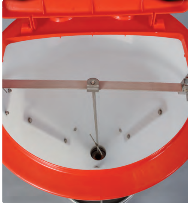
The interior construction prevents a formation of bridges
