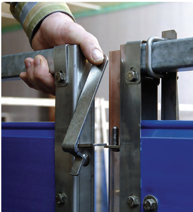
Problem-free one-handed manual opening of the pens is possible.
