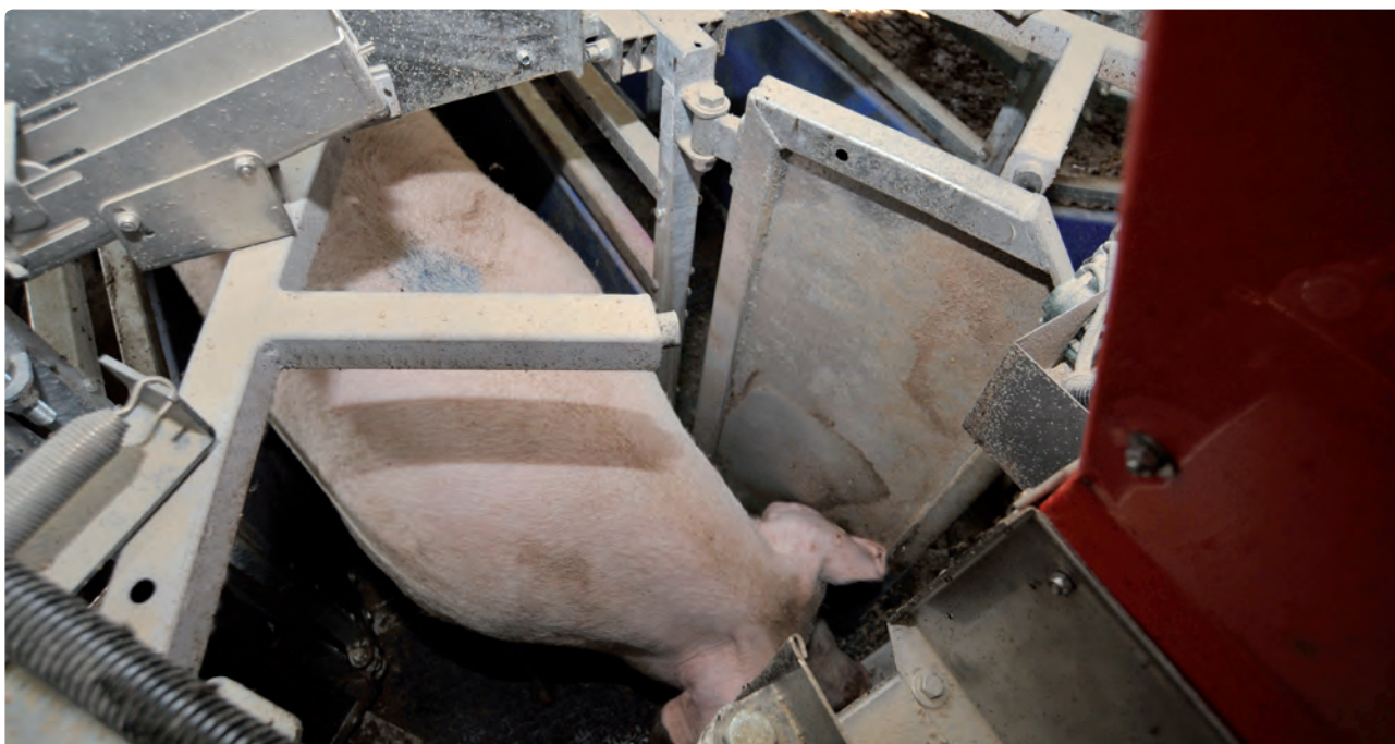
Both entrance gates are alternately opened by the control system.
