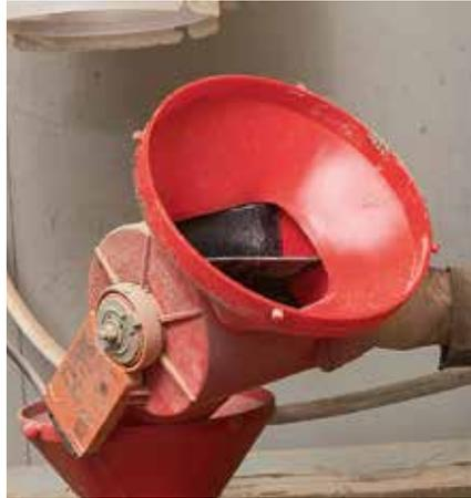
*The cell wheel meters and dispenses only a small and precisely defined quantity of feed.*
