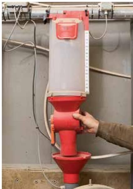
*The feed drops from the removable cell wheel through a funnel into the downpipe.*
